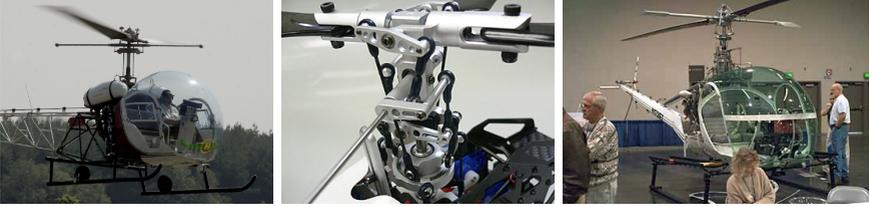
**Figure 4.3:** The Bell stabilizer bar (left)(Source: <http://www.zap16.com>), the Hiller paddle auxiliary rotor (center)(Source: <http://www.copters.com>) and the Bell-Hiller system (right)(Source: <http://www.rclineforum.de>).
