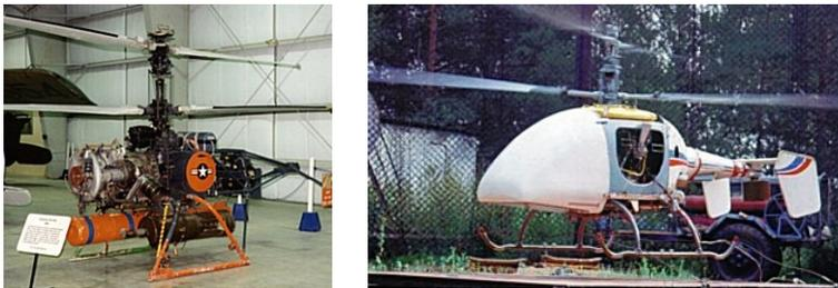
**Figure A.7:** Coaxial helicopter UAVs: the Gyrodyne QH-50 (left) and the Kamov Ka-37 (right).
