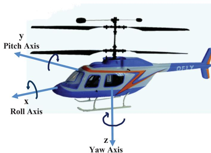
**Figure 2.2:** Body axis system used in helicopter dynamics analysis
