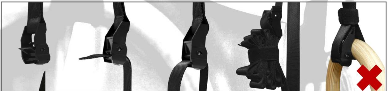
**Step 1:** Feed the strap from below through the quick-release fastener by pressing the buckle downwards.
